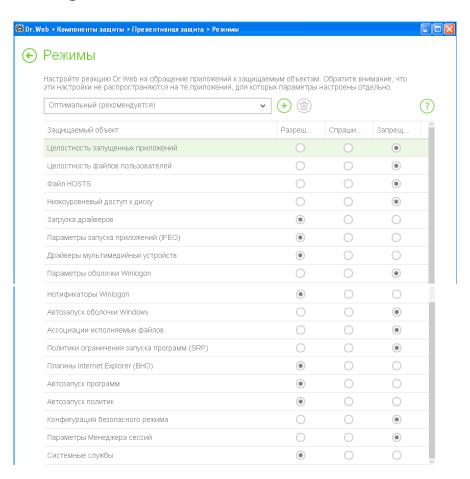
In the default **Optimal** mode, the automatic modification of system objects—activity that would clearly indicate malicious activities are occurring in the system—is disabled. Low-level access to the disk is also disabled to protect the system from bootkits and blocker Trojans that infect the Master Boot Record. So that malware cannot prevent the anti-virus from being updated via the Internet or block access to anti-virus developers' sites, modifying the HOSTS file is not allowed.
